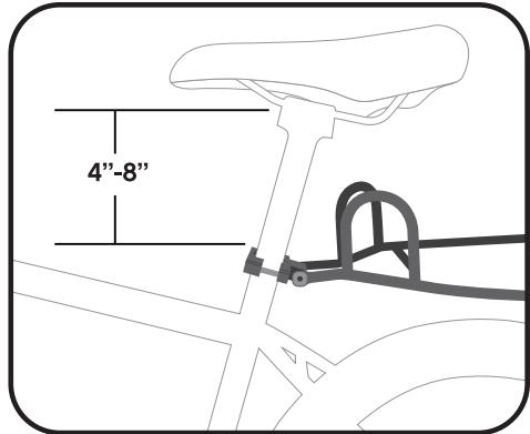
2. Loop the middle strap through both rails of your saddle and snap into buckle. The strap should hang loosely.
