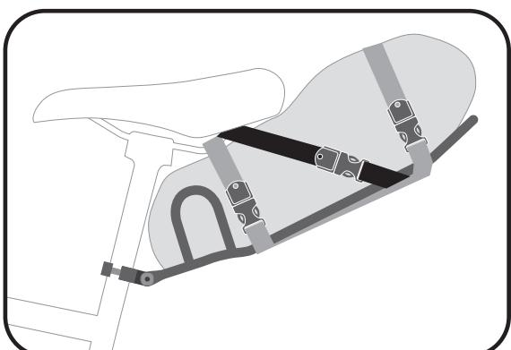
**Warning:** Always check the security of the Bindle hardware and buckles before use. Do not use if bolts or straps are loose.
