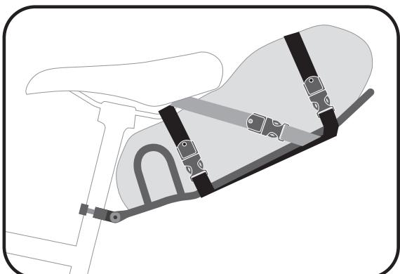
4. Adjust the middle strap to pull the load up securely under your saddle.
