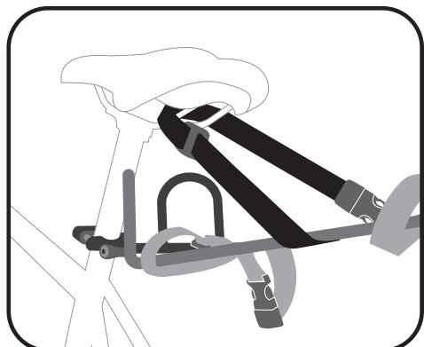
3. Place drybag or other gear onto the Bindle platform, making sure the load is pushed all the way forward to the rack guards. Secure load by tightening the front and rear compression straps.
