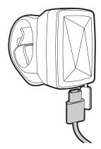
Plug smaller end of USB cable into the Asteroid™ and the other end into a USB port on a computer or wall socket adapter.
