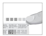
You will then be able to read the degree of water hardness from the discoloration of the Aquadur<sup>®</sup> test strip and the description on the packaging.
