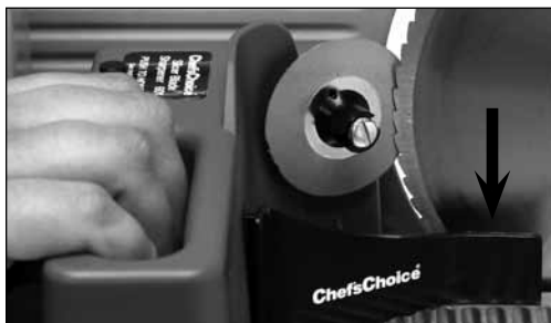
Figure 8. Slicer blade should contact sharpening disk as shown.
