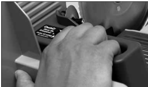
Figure 6. Move food carriage forward to position sharpening disk behind the slicer blade as shown.
