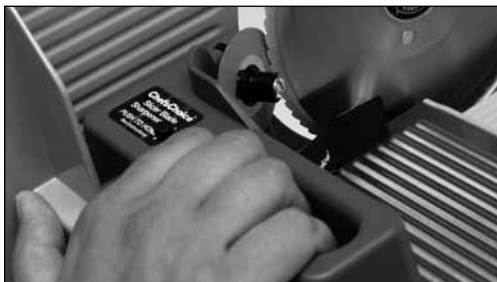
Figure 7. Move sharpening disk into contact with its blade edge.
