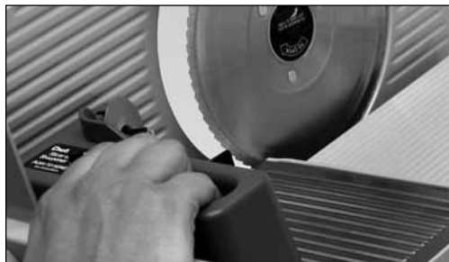
Figure 5. Slide blade sharpener against thickness control plate (shown fully open).
