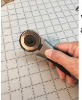
When you want to open the blade press the button with your thumb and hold the button in the down position.
