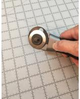
Now <u>gently</u> push the blade down on the cutting mat (still keeping the button pushed down) and the blade will be exposed. Release the button and the blade will stay locked in the exposed position.
