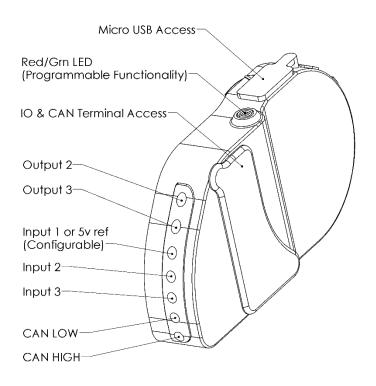
**Plain English:** The Control Module is a programmable relay controller that can control up to three relays. It accepts three analog inputs and has a single CANbus. Outputs are fully programmable based on any configuration of inputs.
