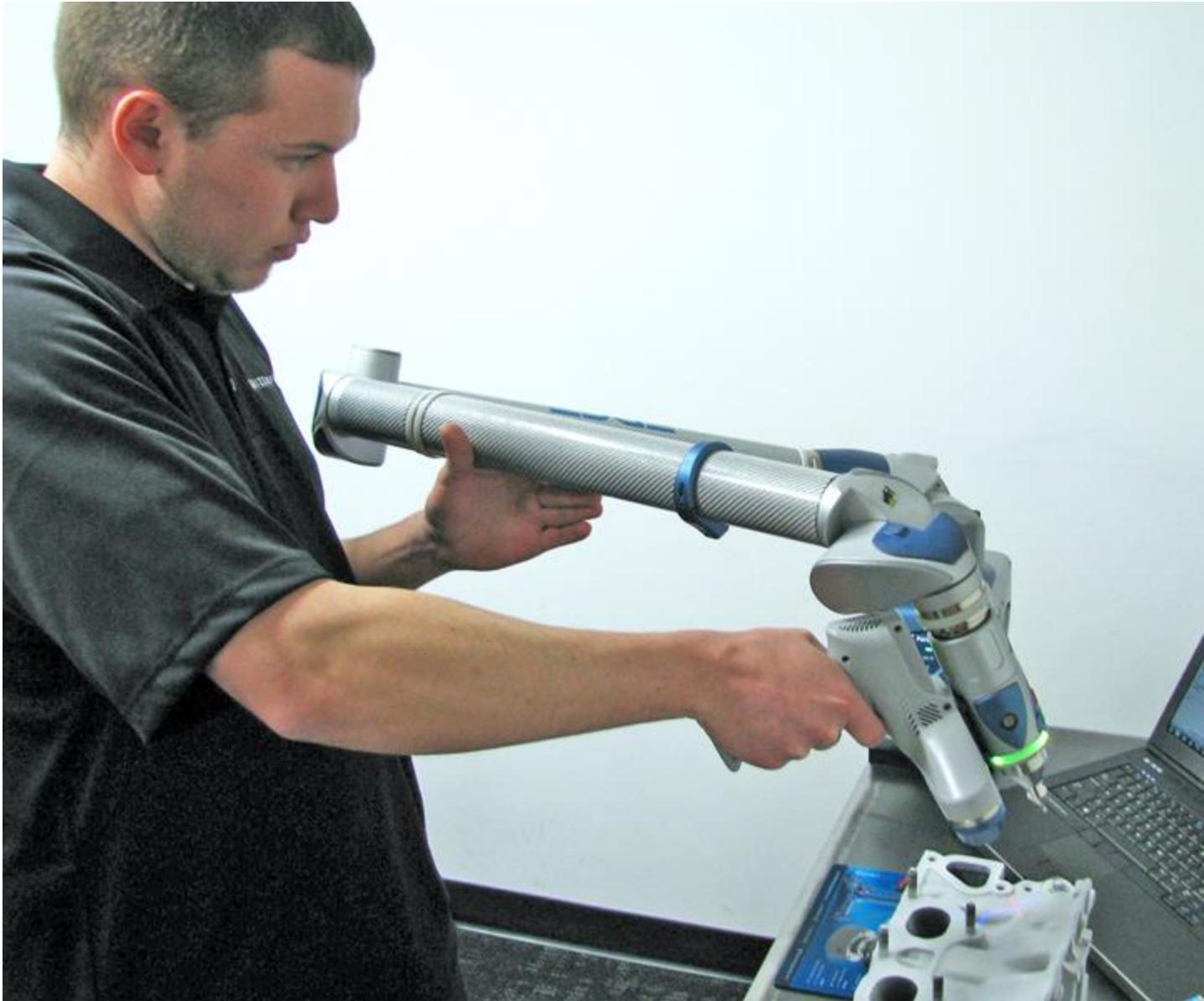
*Brandon Vazquez, KAIZENSPEED's research and development engineer, uses the FaroEdge to make a 3-D scanned image, providing a platform for designing parts that fit precisely. The process that previously took two weeks to complete can now be done in eight hours and is accurate to .002 of one inch over a 9-foot span.*
