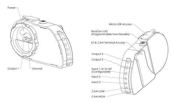
The Smoothboost Controller interfaces with the factory powertrain CANbus using a Kaizen Relay and Control Module. We use parameters such as Front and Rear Wheel Speed, Throttle Position, Engine RPM and others to providing varying duty cycle outputs to get your car hooked up and down the track as quickly as possible.
