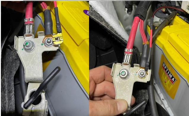
4. Attach the chassis ground loop to the chassis and mount the Kaizen Relay assembly.
