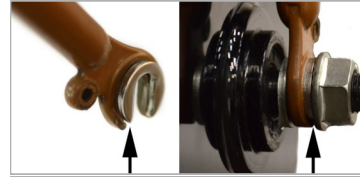
Put the c-washer inside the QR tabs
