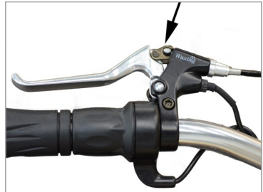
Make sure the E-Brake is closed
