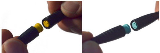
Just unplug the cable to disable throttle or PAS
