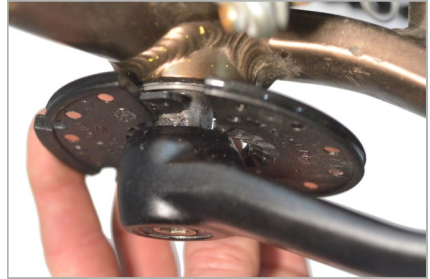
Push the two halves together
