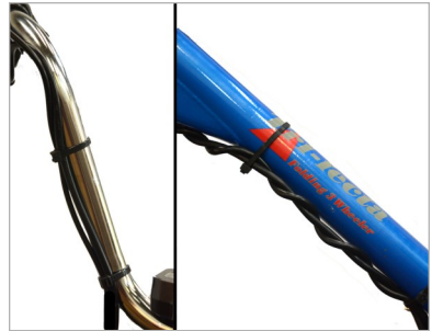
Secure the wires with zip ties
