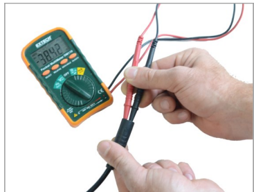
Test the battery voltage.
