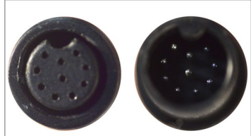
Check for bent pins
