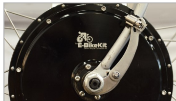
Connect the arm to axle and frame
