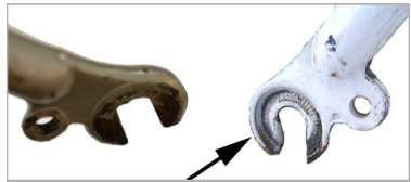
Quick release tabs (right) and none (left) Left dropout filed to fit axle (see below)
