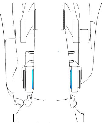
11. Install the outer 1.5 X 19mm inner diameter o-rings over the pivot caps as shown:
