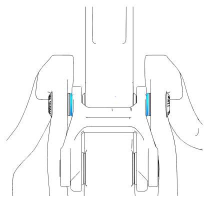
6. Install the inboard 1.5 X 13mm inner diameter o-rings over the pivot bolts:
