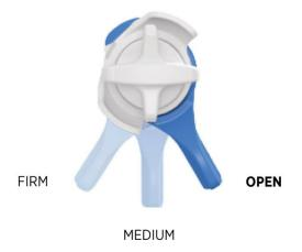
**Open Mode Adjust**: Open mode adjust is useful to control shock performance during rider weight shifts, G-outs, and slow inputs. Open mode adjust provides 3 additional fine tuning adjustments for the OPEN mode. Lift the open mode adjuster, rotate it to the 1, 2, or 3 position, and press it in to lock the position. Setting 1 will have a more plush feel and setting 3 will have a firmer feel.
