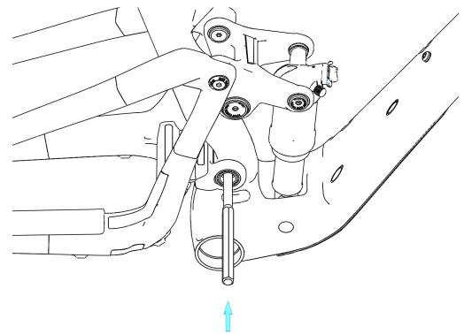
6. The rear triangle is now able to swing upward away from the front triangle. Place a hand under the main pivot yoke while slowly swinging the rear triangle up and rearward to catch the inner pivot washers and o-rings:
