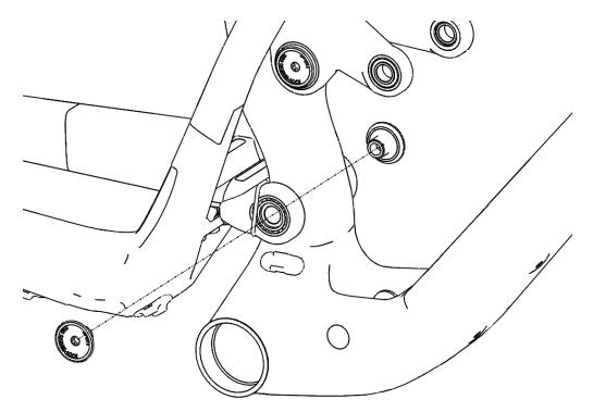
10. Pull the inboard o-rings into place between the pivot clevis and the frame:
