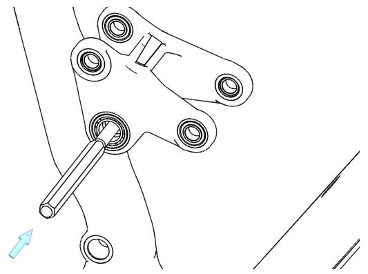
6. The rocker link is now free to slide forward and away from the front triangle. Place a hand under the seat tube pivot to catch the inner pivot washers and o-rings:
