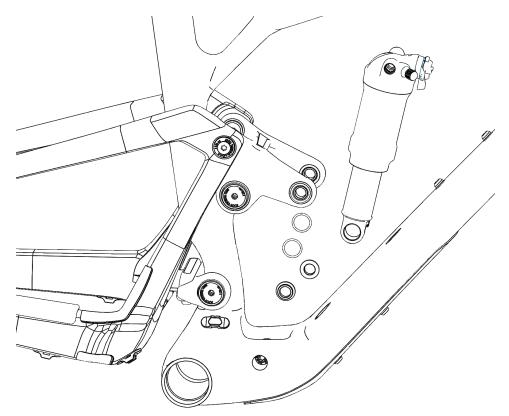
5. To replace the rear shock, begin by fitting new 1.5 X 13 inner diameter EPDM o-rings onto the washers as shown. The easiest way to do this is to lay the washer on a flat surface with the flat side down. Then push the o-ring down from the top until it sits in the installation groove:
