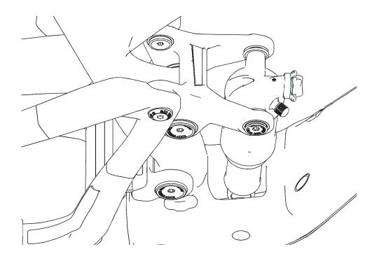
7. Using a pick tool or fingernail, push the inboard o-rings from the installation groove to the taper so they rest against the inboard sides of the link. Install the outboard 1.5 X 13 inner diameter o-rings over the heads of the trunnion screws as shown:
