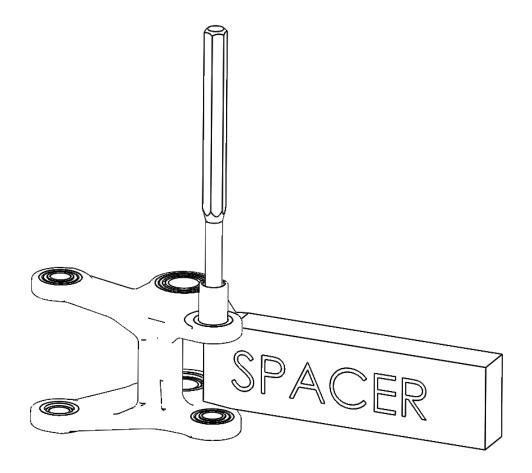
4. Once the old bearings are removed, thoroughly clean the bearing bores in the rocker link with isopropyl alcohol. Similar to the main pivot bearings, there are a few different techniques that can be used for installation. We recommend using an arbor press, but a bench vise, or even a piece of threaded rod with nuts and washers on either end will do the job. Press the bearings until they reach the bottom of their bores, taking care not to mar the finish of the link:
