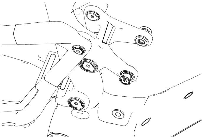
6. Insert the rear shock into the frame and tighten the upper trunnion screws and lower pivot pin hardware to 11N-m (97in-lb) using T30 Torx tools:
