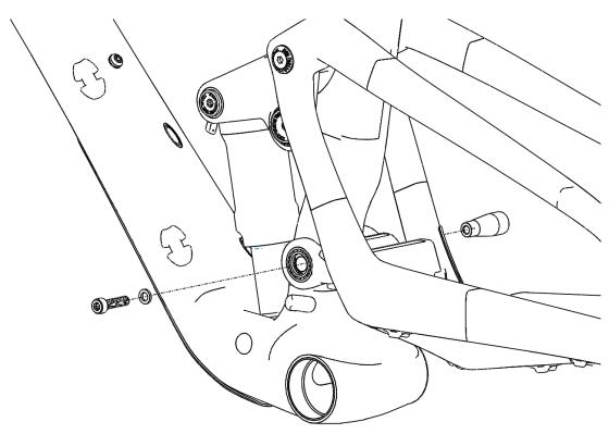
Insert the punch tool into the main pivot bore from where the drive side pivot axle was removed. Ensure firm, even contact with the inner face of the non-drive side pivot axle. Strike the punch sharply with a hammer to unseat the non-drive side pivot axle and remove:
