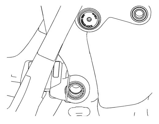
9. Insert the pivot axles, washer and preload screw into the main pivot as shown. Note that the drive side pivot axle is longer than it's corresponding part used in the seat tube pivot. Do not apply thread locker to the preload screw, do not grease the conical axles. Torque to 10N-m (88in-lb) using a T30 Torx tool:
