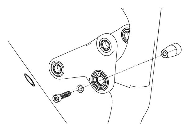
5. Insert the punch tool into the seat tube pivot bore from where the drive side pivot axle was removed. Ensure firm, even contact with the inner face of the non-drive side pivot axle. Strike the drift punch sharply with a hammer to unseat the non-drive side pivot axle and remove:
