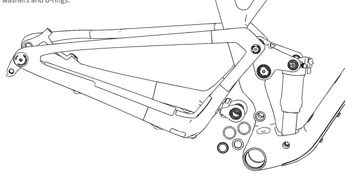
7. Remove the upper pivot hardware from the seat stay / rocker link pivot using T30 Torx tools. The inboard o-rings will come off with the upper pivot bolts:
