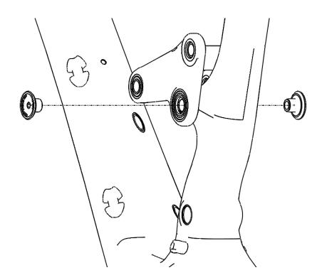
5. Using a pick, small screwdriver, or even a fingernail, move the inner o-rings from the installation groove outward into the sealing position against the link as shown here:
