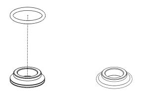
6. Apply medium strength thread locker to the trunnion screws and insert them into the link so that they slightly protrude to the inboard side. Slide the washers, with o-rings, onto the ends of the screws from the inboard side:
