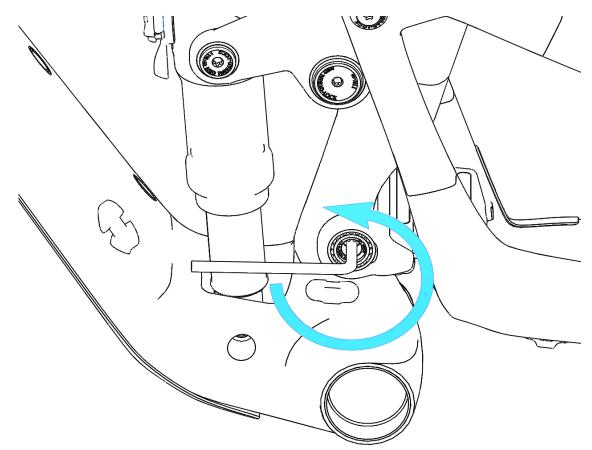
3. Position a the pin punch tool against the head of the preload screw, and sharply strike the punch tool with a hammer to unseat the pivot axle on the drive side of the frame:
