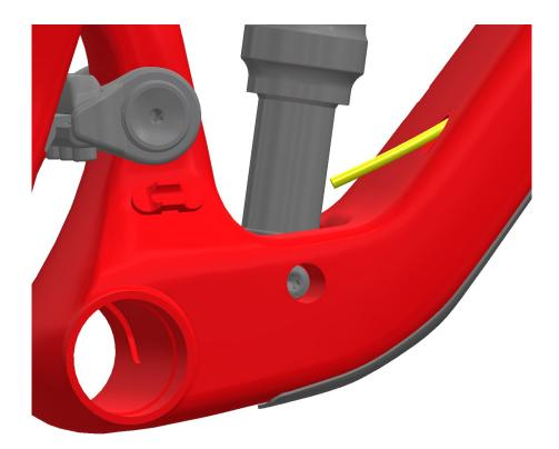
2. Continue routing the cable, affixing it to the guides with zip ties. Begin with the first one just below the main pivot, then proceed along the lower edge of the drive side chain stay:
