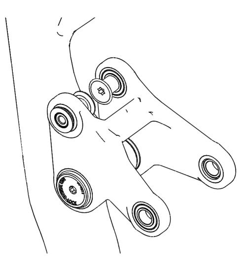
3. Slide the rear triangle assembly onto the upper pivot of the link:
