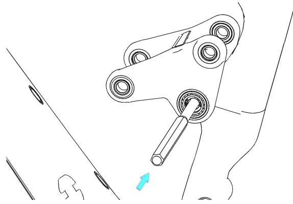
4. Unscrew the preload screw from the drive side pivot axle and remove the screw, washer and axle from the frame:
