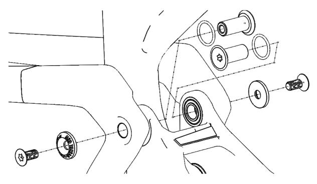
8. Once the upper pivot bolts are removed, the rear triangle assembly can be separated from the frame. Place a hand under the upper link while pulling the rear triangle rearward to catch the inner washers and o-rings from the upper link:
