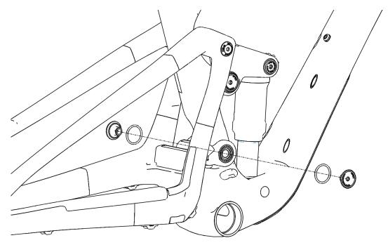
2. Using a T30 Torx tool, loosen the preload screw from the pivot axle 5-6 full turns:
