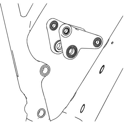
3. Insert the pivot axles, washer and preload screw into the seat tube pivot as shown. Note that the drive side pivot axle is shorter than it's corresponding part used in the main pivot. Do not apply thread locker to the preload screw, do not grease the conical axles. Torque to 10N-m (88in-lb) using a T30 Torx tool:
