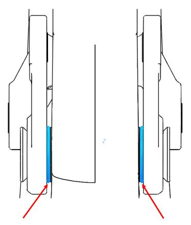
6. Install the outer pair of o-rings (1.5 X 19mm inner diameter):
