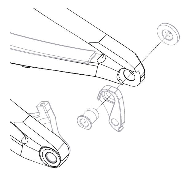
The derailleur hanger is removed using a 8mm hex tool on the outboard cap. Turn the cap counter-clockwise to unscrew, then remove the axle sleeve and hanger from the inboard side. When replacing the derailleur hanger, be sure to orient the flat section of the axle sleeve flange downward to match the opening in the hanger. Apply medium strength (blue) thread locking compound to the cap. Torque: 8.0Nm (71in-lb)
