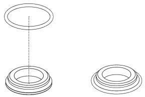
2. Insert the washers, with o-rings positioned in the installation grooves, into the inboard lower bearing recesses on the link assembly. A small application of grease can help to keep them in place for link installation. Being careful not to drop the washers/o-rings, and carefully slide the link assembly rearward onto the seat tube at the pivot boss::
