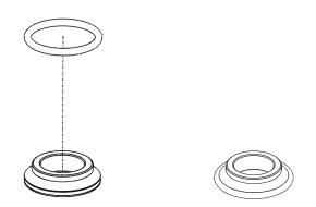
2. Insert the upper pivot axles into the link from the inboard side so that they slightly protrude to the outboard side. Slide the washers, with o-rings, onto the ends of the axles from the outboard side:
