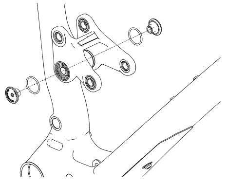
2. Using a T30 Torx tool, loosen the preload screw from the pivot axle 5-6 full turns:
