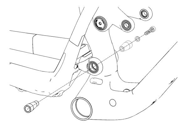
10. Install the two outer pivot caps as shown. Apply medium thread locker and torque to 11N-m (97inlb) using a T30 Torx tool:
