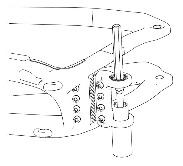
2. Remove the remaining main pivot bearing by flipping the rear triangle over and repeating.
