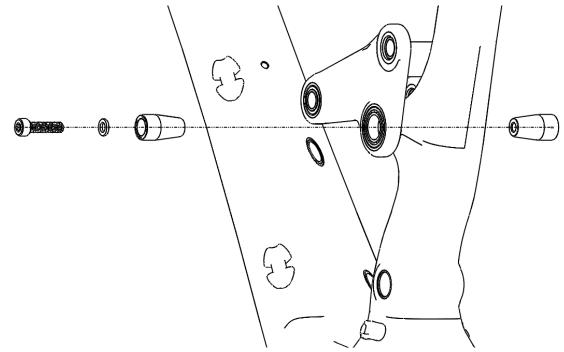
4. Install the two outer pivot caps as shown. Apply medium thread locker and torque to 11N-m (97in-lb) using a T30 Torx tool:
