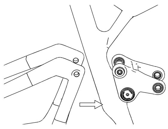
4. Install the upper pivot screws and washers with medium strength thread locker. Torque to 11N-m (97 in-lb) using T30 Torx tools:
