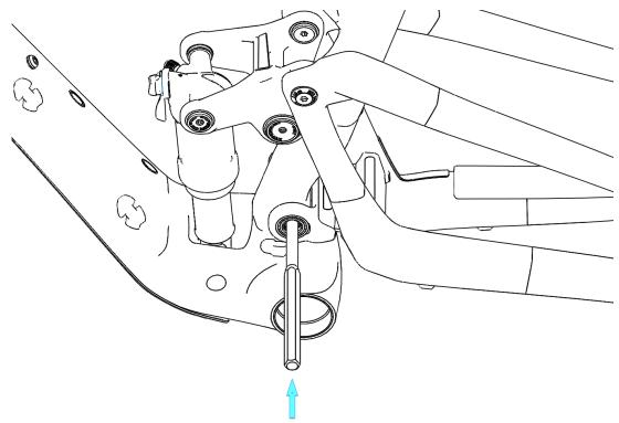
4. Unscrew the preload screw from the drive side pivot axle and remove the screw, washer and axle from the frame:
