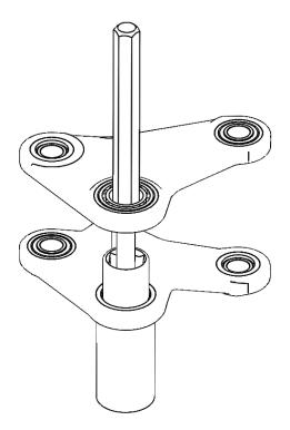
2. The shock bearings in the link are removed in the same manner, but require smaller 13-14mm socket and 23-25mm ID tube.
