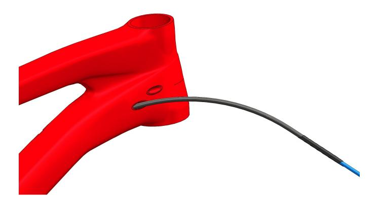
4. Proceed to install your dropper seatpost per the seatpost manufacturer's instructions. *You may wish to install other components on the frame before completing the dropper post instal-lation.*
