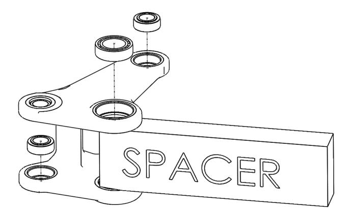
When pressing in bearings from the outboard side of the link, be sure to support the link with some kind of spacer block to prevent link damage.
