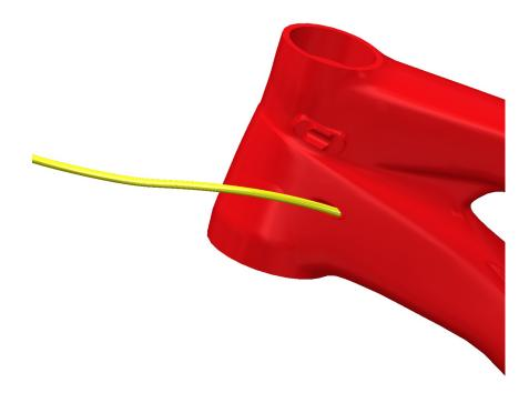
2. The housing will emerge from the corresponding port atop the down tube above the bottom bracket area:
