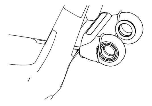
8. Swing the rear triangle into place aligning the clevis to the main pivot:
