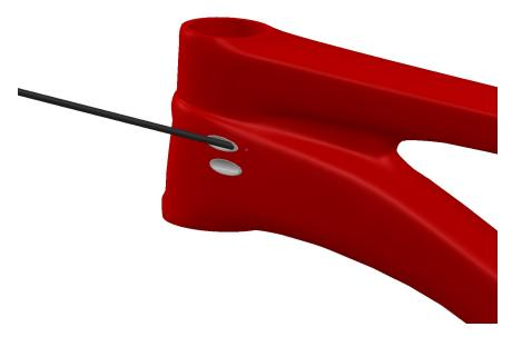
2. The housing will emerge from the corresponding port behind the seat tube, just above bottom bracket.
