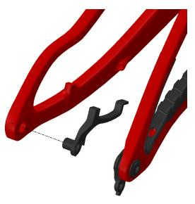
2. If the lever is connected to the hose, cut the hose close to the lever and plug. Follow manufacturer recommendations for plugging/capping the brake hose before internally routing. Once the hose is plugged, begin feeding the brake hose into the port on the non-drive side chainstay.
