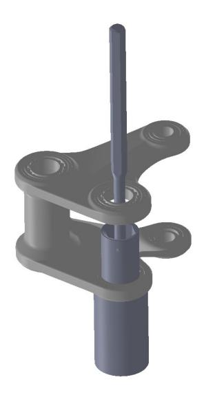
2. The shock bearings in the link are removed in the same manner, but require smaller 13-14mm socket and 23-25mm ID tube.
