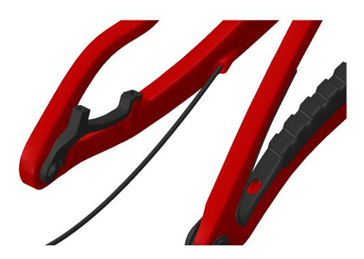
3. The brake hose will exit the non-drive side port at the front of the rear triangle. With the upper shock hardware removed, swing the rear triangle forward to give more space in between the front and rear triangle. Feed the brake hose into the non-drive side port on the front triangle just above the bottom bracket.
