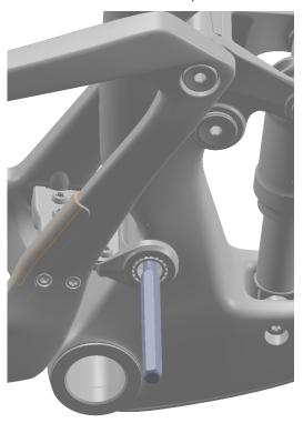
6. The rear triangle is now able to swing upward away from the front triangle. Place a hand under the main pivot yoke while slowly swinging the rear triangle up and rearward to catch the inner pivot washers and o-rings:
