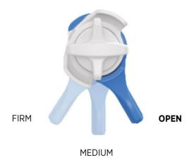
**Open Mode Adjust**: Open mode adjust is useful to control shock performance during rider weight shifts, G-outs, and slow inputs. Open mode adjust provides 3 additional fine tuning adjustments for the OPEN mode. Lift the open mode adjuster, rotate it to the 1, 2, or 3 position, and press it in to lock the position. Setting 1 will have a more plush feel and setting 3 will have a firmer feel.
