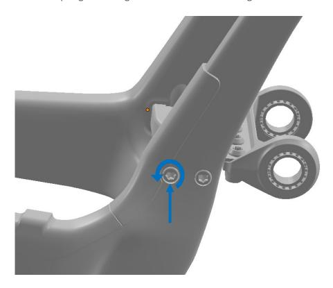
4. Slide the rear triangle assembly onto the upper pivot of the link. Be careful when sliding the seatstays over the link, as it may be necessary to lightly spread the pivot points apart to fit over the washers.
