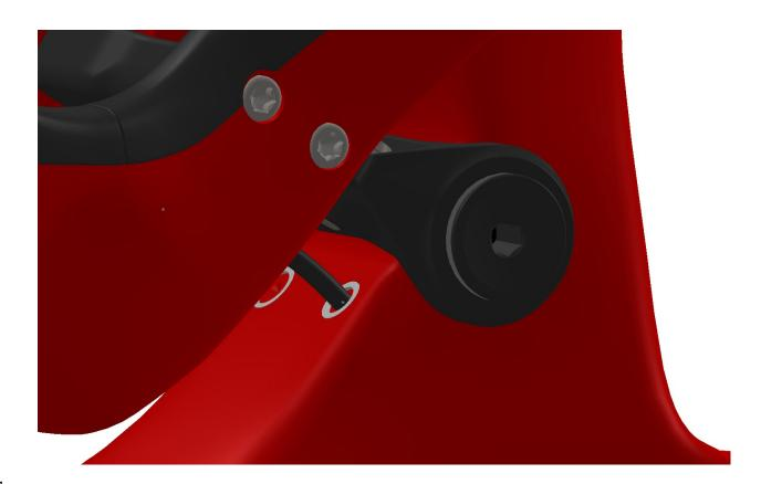
2. Insert the housing into the drive side port on the rear triangle. The housing will exit the rear triangle at the drive side chain stay.
