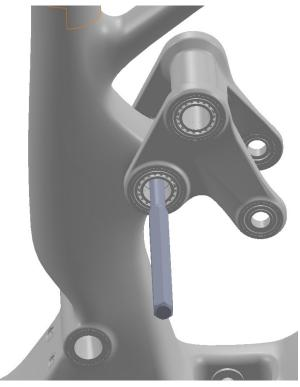
6. The rocker link is now free to slide forward and away from the front triangle. Place a hand under the seat tube pivot to catch the inner pivot washers and o-rings:
