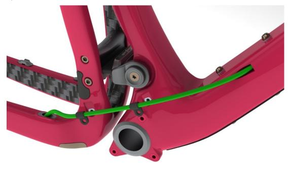
4. Feed the cable housing though the headset until desired length is reached. Then secure p-clips to the frame as shown below.
