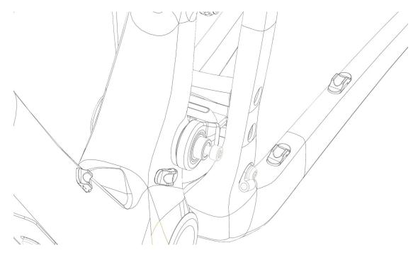
4. Sharply strike the head of the center screw with a hammer. A drift punch can be used here to improve hammer accuracy. This will unseat the pivot axle on the drive side from its taper. Remove the center screw and drive side pivot axle:
