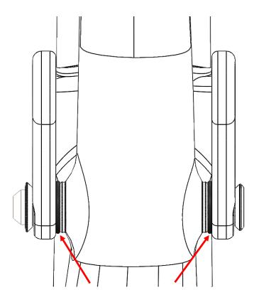
6. Install the outer pair of o-rings (1.5 X Ø13mm):
