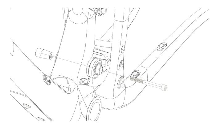
5. Insert an Ø8-10mm drift punch into the main pivot bore from where the drive side pivot axle was removed. Ensure firm, even contact with the inner face of the non-drive side pivot axle. Strike the drift punch sharply with a hammer to unseat the non-drive side pivot axle:
