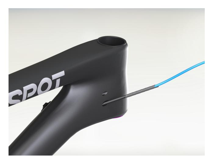
4. Proceed to install your dropper seatpost per the seatpost manufacturer's instructions. You may wish to install other components on the frame before completing the dropper post installation.
