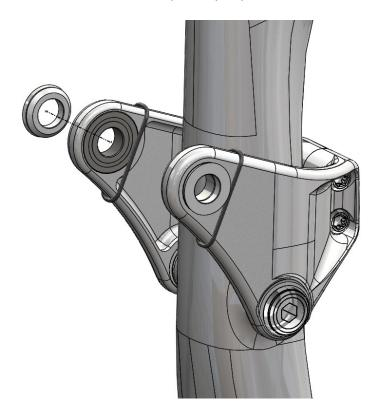
3. Slide the rear triangle assembly onto the upper pivot of the link:
