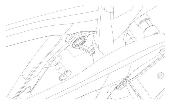
8. Once the upper pivot bolts are removed, the rear triangle assembly can be separated from the frame. Place a hand under the upper link while pulling the rear triangle rearward to catch the inner washers and o-rings from the upper link:
