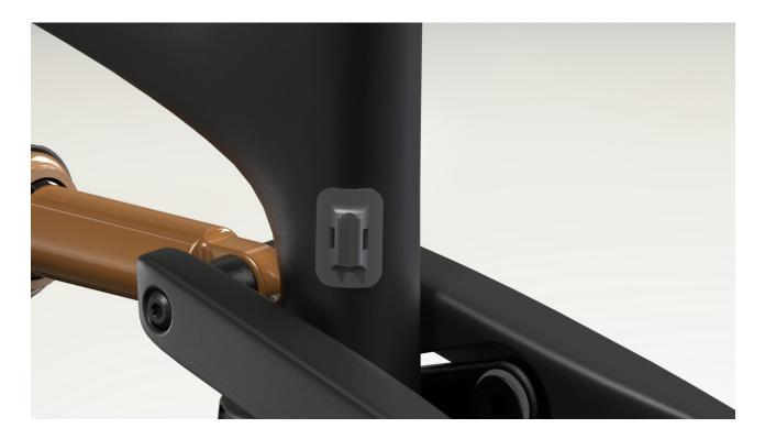
2. The external seatpost cable/hose will share cable saddles on the down tube. Route and attach the line as shown:
