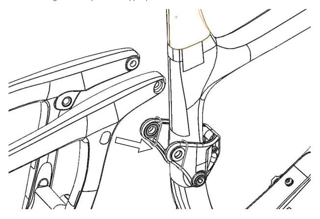
4. Install the upper pivot bolts with medium strength (blue) thread locker. A bit ratchet with 6mm bit is very handy here. Torque to 9Nm (80in-lb):
