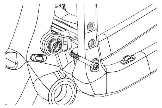
10. Pull the inboard o-rings into place between the pivot clevis and the frame:
