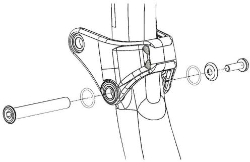
2. Gently slide the upper link assembly forward, keep a hand beneath the link assembly to catch the inner washers and o-rings:
