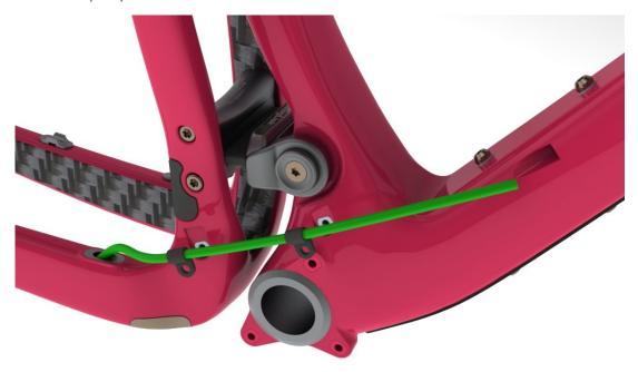
3. Feed the cable housing into the port on the drive side of the down tube. It will emerge from the port on the non-drive side of the head tube:
