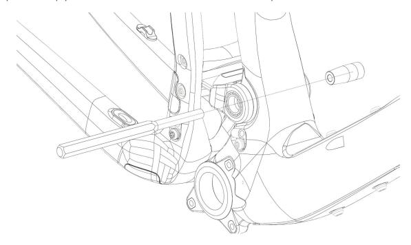
6. With the rear shock assembly removed from the frame, the rear triangle is now able to swing upward away from the front triangle. Place a hand under the main pivot yoke while slowly swinging the rear triangle up and rearward to catch the inner pivot washers and o-rings:
