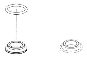
2. Insert the washers, with o-rings positioned in the installation grooves, into the inboard lower bearing recesses on the link assembly. A small application of grease can help to keep them in place for link installation:
