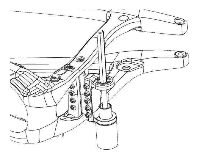
2. Remove the remaining main pivot bearing by flipping the rear triangle over and repeating.
