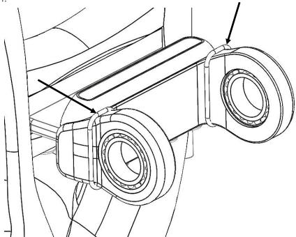
8. Install the inner washers, with the conical faces outboard—flat faces inboard, into the inboard bearing recesses in the main pivot clevis. The o-rings will help hold the washers in position and vice versa. A small dab of grease on each washer can help it stay in place for installation. Swing the rear triangle into place aligning the clevis to the main pivot:
