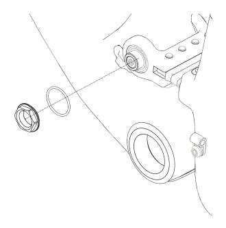
3. Using a T30 Torx tool, loosen the center screw until the head stands 10mm above the surface of the pivot axle:
