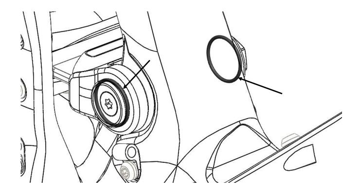
13. Install the shock unit. Torque fasteners to 8.5Nm (75in-lb):
