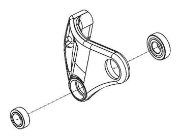
2. Reassemble the upper link using the two T30 Torx screws and medium strength (blue) thread locker. Torque to 8.5Nm (75in-lb):
