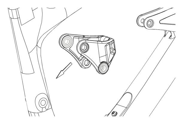
4. Reinstall the pivot axle, washer, and screw. Apply medium strength (blue) thread locker to the T25 Torx screw and torque to 8.5Nm (75in-lb):
