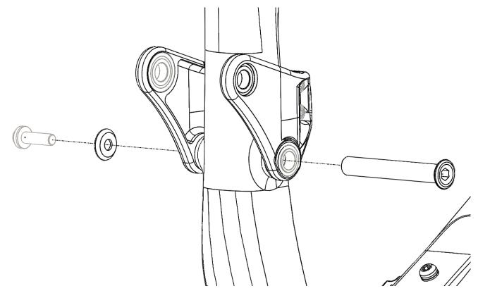
5. Using a pick, small screwdriver, or even a fingernail, move the inner o-rings from the installation position outward into the sealing position as shown here:
