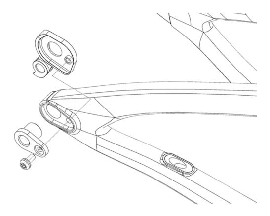
2. The derailleur hanger is removed using a T25 Torx tool on the external screw. When replacing the derailleur hanger, be sure to apply medium strength (blue) thread locking compound to the screw. Torque: 6.5Nm (57in-lb)
