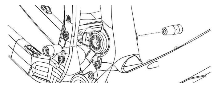
IMPORTANT: DO NOT GREASE CONICAL SURFACES OF PIVOT AXLES OR BORES IN FRAME! GREASE CAN ALLOW TOO MUCH FORCE IN THE FRAME FOR THE SPECIFIED TORQUE VALUE AND DAMAGE THE FRAME!
