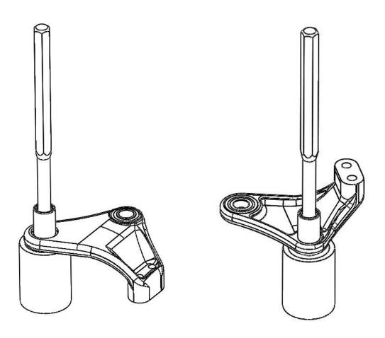
2. The lower bearing in the link is removed in the same manner, but is pressed outward, away from the centerline of the frame.
