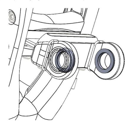
8. Clean the two conical main pivot axles with alcohol before inserting into their bores in the frame. The longer, externally threaded axle goes in the non-drive side, and the shorter, internally tapped axle goes into the drive side:
