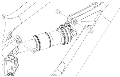
5. Installation is the reverse of removal. Pivot fastener torque: 8.5Nm (75in-lb)
