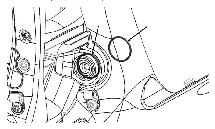
11. Install the outer nut (19mm hex) on the non-drive side and pivot cap (T30 screw) on the drive side. Apply fresh medium strength (blue) thread locker to the nut and screw for installation. Torque: 6.5Nm (57in-lb) both sides:
