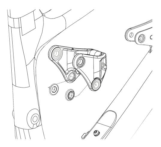
3. Being careful not to drop the washers/o-rings, and carefully slide the link assembly rearward onto the seat tube at the pivot boss:
