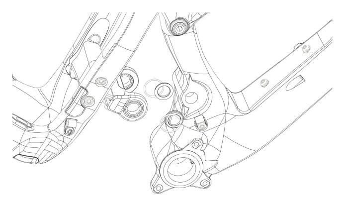
7. Remove the upper pivot bolt from inside of each shock stay at the upper link using a 6mm allen wrench, or better yet, a bit ratchet with a 6mm hex bit. The o-rings will come off with the upper pivot bolts:
