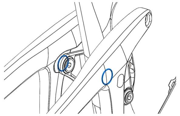
6. Install the inboard o-rings over the pivot bolts:
