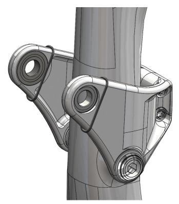
2. Install the upper washers, with the conical faces inboard– flat faces outboard, into the bearing recesses in the upper link. The o-rings will help hold the washers in position and vice versa. Again, a small dab of grease on each washer can help it stay in place for installation:
