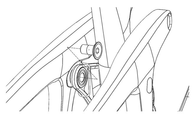
5. Pull the outboard o-rings over the "ears" of the link to set them into position between the link and the shock stays:
