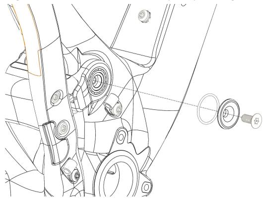
2. Using a 19mm open end wrench, remove the non-drive side pivot nut and o-ring:
