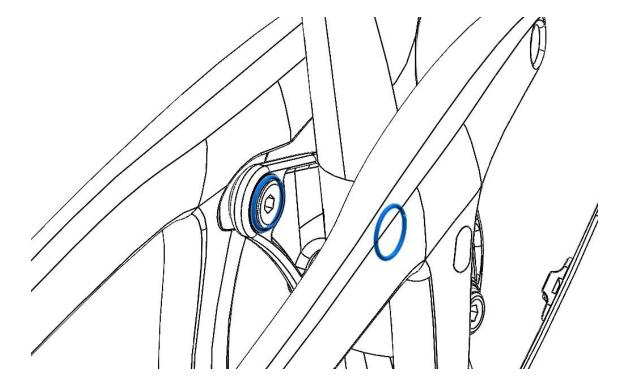
7. Stretch two lower o-rings (1.5 X Ø19mm) over the hoops of the main pivot bearings to prepare for installation:
