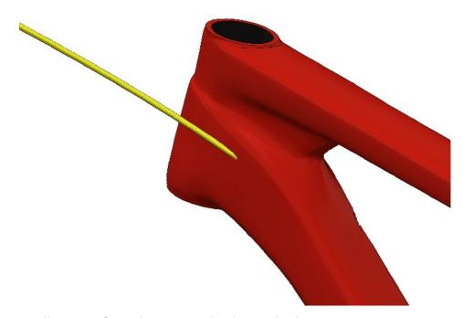
2. The housing will emerge from the port on the drive side chainstay:
