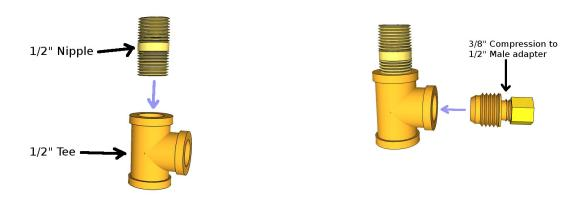
Next thread the two assemblies into the hot and cold port of the water heater.
