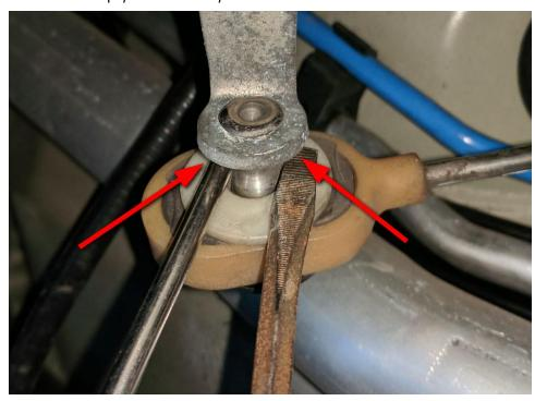
4. With the DEM cable end free from the transmission, you can now remove the internals. **Be sure to wear safety glasses**. Snip away the top portion of the inner plastic disc with the dikes (as per the dotted line), taking care to not damage the surrounding plastic frame, and push the internals through the frame. For the next steps, be sure to keep track of which side of the cable end faces the transmission.
