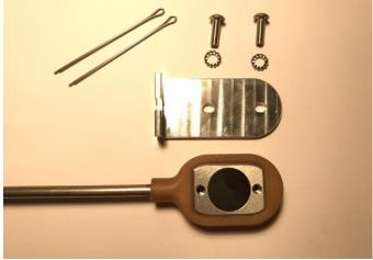
6. Slide the half-circle cutout of the top cover over the shifter cable, and butt it up against the base of the shifter cable end frame, ensuring there is no gap, while you fully tighten the 2 button head screws with locknuts.
