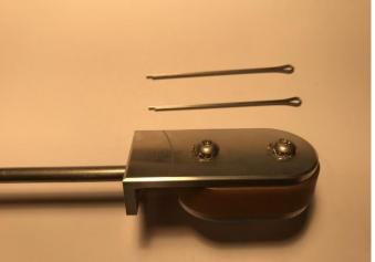
NOTE: On the 997 CARRERA models -- the top cover for the "fore/aft" shifter cable (the cable that connects to the gear selector arm with the counterweights) needs to be installed BACKWARDS, as shown in the below picture:
