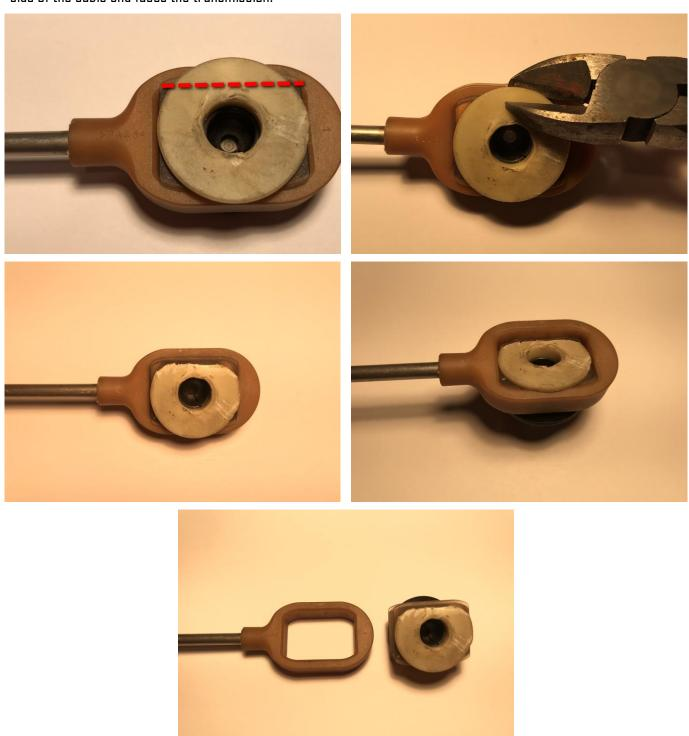
5. If not already done so, pre-assemble the new cable ends. Place the stainless steel ring clip into the recess of the aluminum receiver, then slide the cupped side of the Delrin bushing on top. Press the completed receiver assembly into the shifter cable end frame, **FROM THE INSIDE** (btwn transmission and cable) **TOWARD THE OUTSIDE**.
