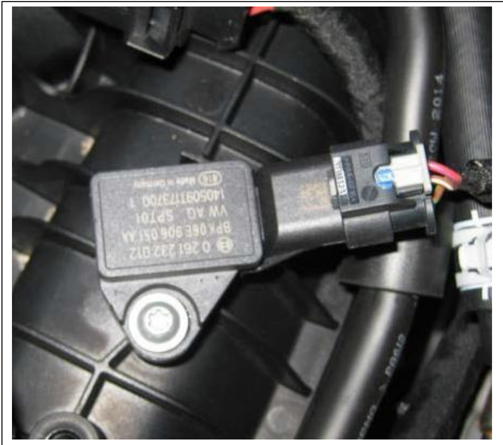
Detailed view on Turbo charger sensor (3-pin) placed behind the front mask:
