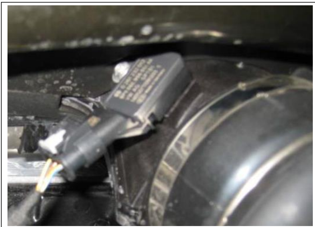
Detailed view on Turbo charger sensor (3-pin) placed behind the front mask:
