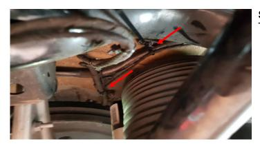
**Step 2)** The Can-Bus must be laid in the "center".
