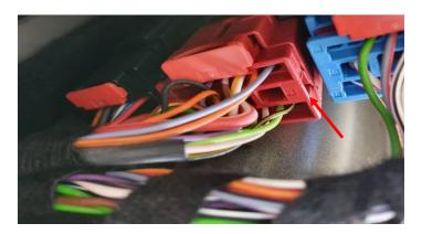
It is important that you press the adapter (Can-Bus connector) together with a pair of pliers so that contact is made.
