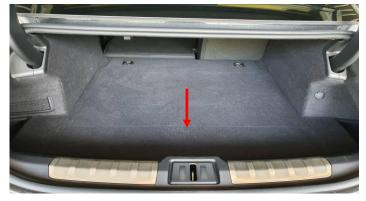
**Step 3)**Open the trunk and remove the bottom cover.
