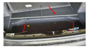
**Step 5)**Dismantle the load compartment cover.
