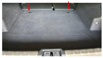
**Step 4)**Remove the necessary screws to be able to remove the rail.
