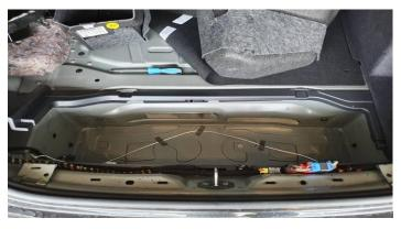
**Step 6)** In order to get the can line inside, the grommets in the trunk floor could be used, for example.
