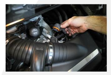
4. Disconnect the solenoid plug from the right-rear of the air box.
