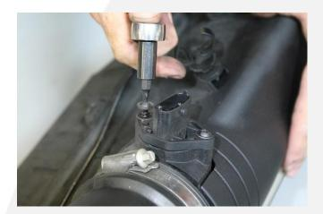
10. Remove the mass airflow sensor.
