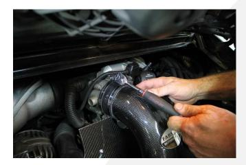
18. Re-connect mass airflow sensor plug.
