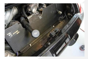
15. Using a 6mm Allen/hex-head wrench, tighten the heat shield bolts into place.
