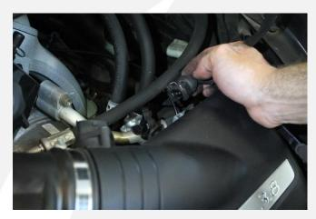
5. Unclip solenoid from the rear of the air box.
