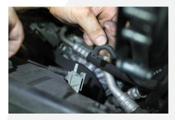
7. Remove the air box from the engine bay and carefully remove the remaining vacuum line from the solenoid. NOTE: If necessary, carefully use a razor blade to break the adhesive seal inside of the rubber fitting.
