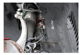
NOTE Once a fitting is loose it will begin to drip and discharge brake fluid. It may be helpful to loosen everything and then quickly swap the lines to minimize the amount of brake fluid being discharged.
