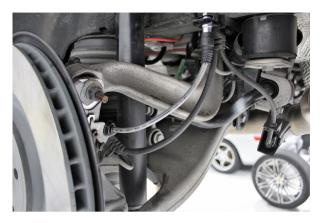
**5**) The front and rear brakes lines are very similar in regard to line layout and mounting brackets. Follow the same procedure at every axle.
