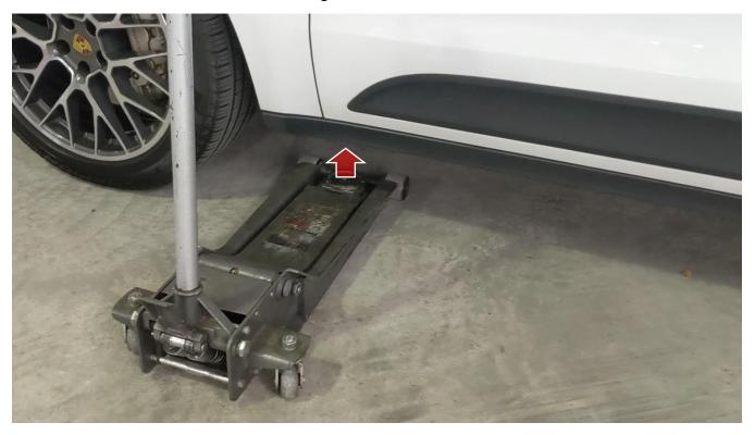
3) With the Macan lifted with both wheels off the ground, remove all 5 wheel-bolts. Please note, the Macan does not use studs so when the final bolt comes off, the wheel will fall. It might be helpful to hold the wheel or place something underneath the wheel to support it to make removal easier.
