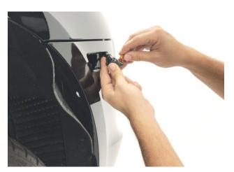
6) Turn the ignition to the "ON" position and make sure your lights illuminate before mounting. Insert the harness socket and turn to tighten (opposite step of removal).
