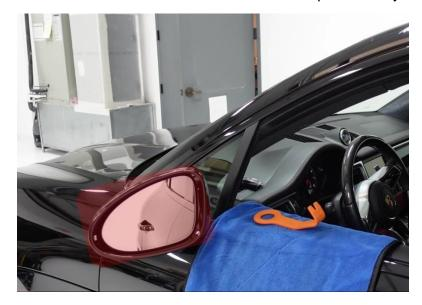
2) Use a trim pry tool to remove the mirror, the mirror is secured in the center of the mirror body, pry and pull straight out.
