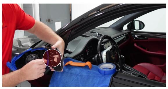
4) Remove the various T-15 & T-25 torx screws securing the mirror body.
