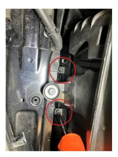
1 4) Using needle-nose pliers or a long T30 bit, rotate the two plastic pins that lock the intake piping to the airbox until the tabs face outwards. They can then be pulled upwards with pliers.
