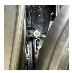
12) Next, move to the passenger side of the vehicle. Looking along the outer edge of the airbox, locate the T30 screw holding the airbox down to the frame rail and unscrew.
