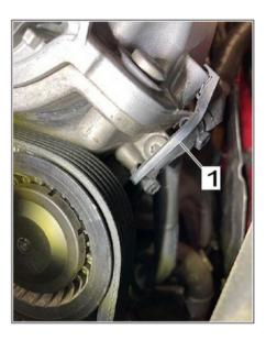
(a) Using a mirror if needed, locate the upper timing cover screw. Once located, gently attempt to unscrew by hand. Rotate very slowly to prevent screw from becoming fully detached. If screw is too tight, you may also loosen with a T30 bit on a small wrench or driver. Be very gentle to prevent further breakage.
