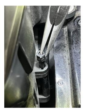
4) Once the pins are removed, use a long flathead screwdriver or suitable tool to pry the intake pipe out of its socket in the airbox. You can now pull the airbox up and out of the engine bay.
