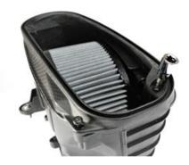
9) Next, install the rubber gaskets on top of the High Flow Carbon Fiber Ducts and ensure they are properly set in the groves. Press firmly on top of the rubber to ensure they are properly seated into the groves.
