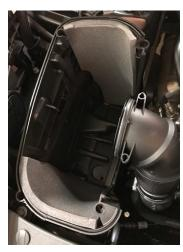
Removal of the factory air filter is now complete, now it's time to install the Flat 6 Motorsports High Flow Air Filter.
