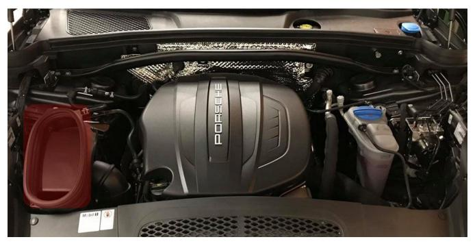
2) Lift up the rubber gasket seals on top of the airbox and place them to the side.
