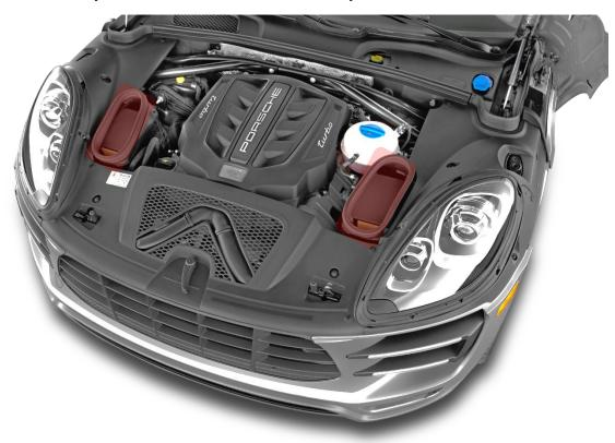
2) Lift up the rubber gasket seals on top of the airbox and place them to the side.
