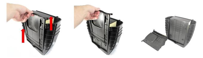
**Note** – The driver's side airbox has a coolant reservoir bleeder valve attached to the air box side panel. This can be removed by simply pulling up on the valve.
