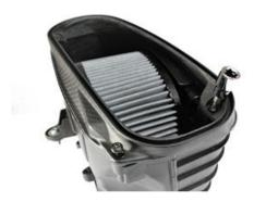
9) Next, install the rubber gaskets on top of the High Flow Carbon Fiber Ducts and ensure they are properly set in the groves. Press firmly on top of the rubber to ensure they are properly seated into the groves.
