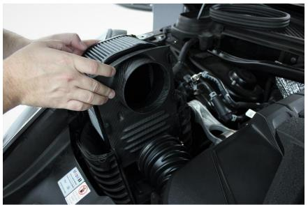
**Note** – There are 6 total retaining clips on the Carbon Fiber Airbox Panel Plate (3 per side), you may need to slightly wiggle to relieve pressure as you slide the filter and panel downward into the airbox.
