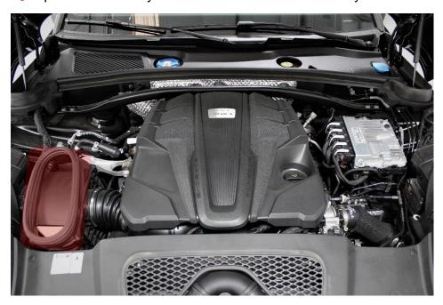
2) Lift up the rubber gasket seal on top of the airbox and place it to the side.Note – you will reuse the gasket on the High Flow Carbon Fiber Duct.
