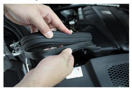
**10)** Align the High Flow Carbon Fiber Duct onto the top of the airbox.
