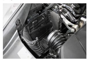
Removal of the factory air filter is now complete, now it's time to install the Flat 6 Motorsports Cold Air Intake System.
