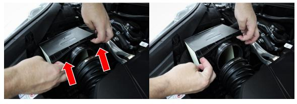
(Image of air filter removed from airbox)
