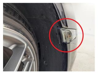
Pull back the fender liner opening and use a flat-head screwdriver and push in the silver release tab to release the side market. It's helpful to use one hand to pry and one hand to help pull the side marker loose. The side marker will release out with a simple press of the release.
