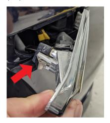
**3**) With the OEM side marker removed, plug in the LED Side Marker to the harness and feed the resistor down into the hole inside of the bumper. Insert the LED Side Marker into the mounting points starting at the front of the light and snap in the rear.
