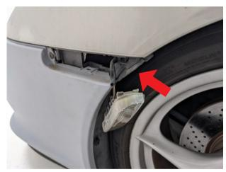
Press the metal retaining clip inward to release the bulb from the side marker housing. Then remove the halogen bulb from the socket by pulling straight outward.
