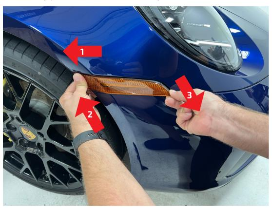
**2)** With the side marker released from the body, disconnect the harness connector by pressing inward on the release tab to disconnect the harness connector from the side marker.
