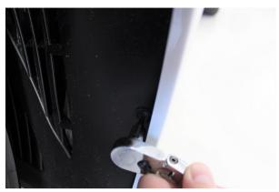
2) Pull back the fender liner opening and use a flat-head screwdriver and push in the silver release tab to release the side marker. It's helpful to use one hand to pry and one hand to help pull the side marker loose. The side marker will release out with a simple press of the release.
