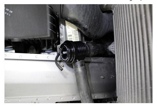
**7)** Use two of the provided worm clamps to secure the diverter valve. Tighten with a flat head screwdriver and ensure the clamps are secure around the diverter valve necks.
