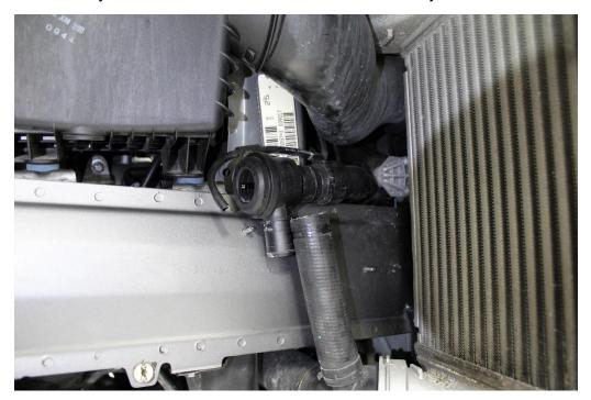
Removal of the factory diverter valve is complete, now it's time to install the Flat 6 Motorsports Upgraded Diverter Valve.
