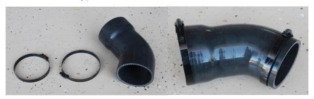
4) Install the provided silicone tube onto the intake box, then slide over the throttle body, ensuring the tube isn't folded onto itself. Tighten clamps to a snug setting.
