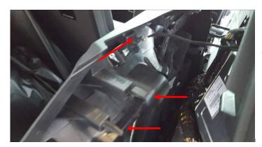
**Step 6)**Now you are able to remove the full cover on the right site. It is clipsed. Take care about connected wires.
