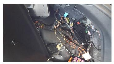
**Step 2)**Please remove the right cover slightly and take care of connected wires.
