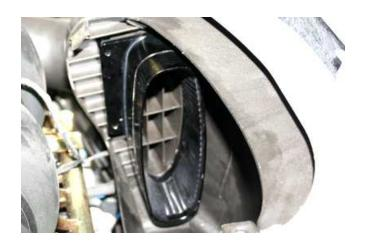
Attach the black V-Flow billet filter collar to the OEM air box by snapping it into the OEM filter port inside of the air box. Make sure that this collar is fully in place before moving on to the next step.
