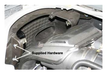
11. Use the supplied hardware to secure the billet filter collar to the OEM air box.
