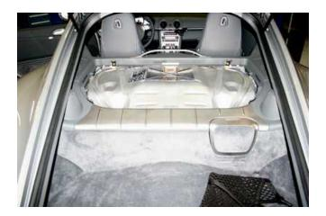
2. Remove the 5, T-30 Torx screws that attach the metal engine cover to the body of the car.
