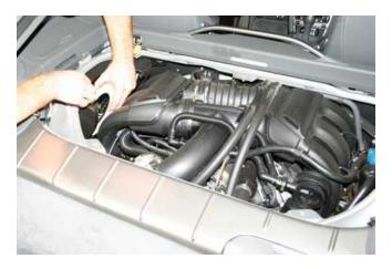
5. Remove the OEM air filter from the car.
