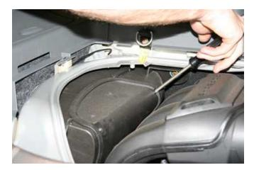
3. Remove the 2, Phillips head screws that attach the air box cover to the air box housing.
