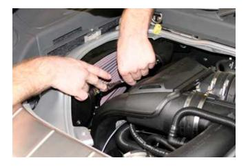
14. Tighten the filter to the collar by tightening the 8 mm hose clamp located on the filter.
