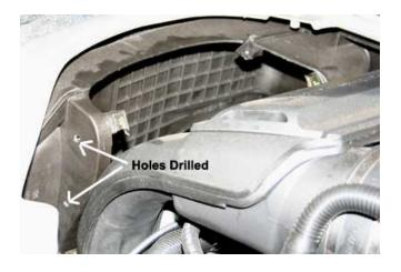
9. Using a 13/64<sup>th</sup> drill bit, drill two holes through the marks made in step 8. Make sure that these holes are drilled as straight and clean as possible.
