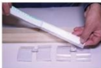
2) Stick it on the rail. 3) Peel the plastic layer of the tape and stick the adhesive on the surface.
