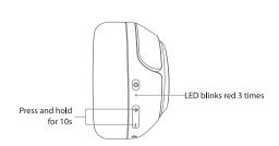
Connected: LED blinks white every 10s Charging: LED glows solid red Top-up: LED glows solid white
