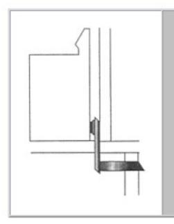
**Figure A:** This installation requires a rectangular hole in the floor for the periscope to pass through. The top portion of the periscope is positioned for attachment to the dryer's exhaust pipe, while the bottom portion of the periscope is attached to the round vent leading to the exterior wall damper.
