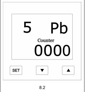
if temperature on heater is higher than circuit board shows,pls lower the Pb value.
