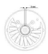
(4) Check electrode connectors (h) be tightened and clean
