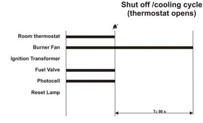
When the heating request (normal operation or thermostat operation) opens:
