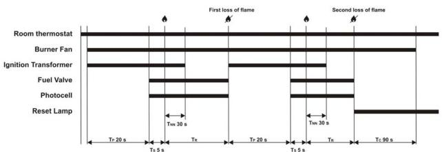
In case of flame failure in running status, the flame control unit make one trial restarting the unit. If the reason of flame failure is confirmed, then the unit stops in lock-out mode, and the reset lamp becomes steady red.
