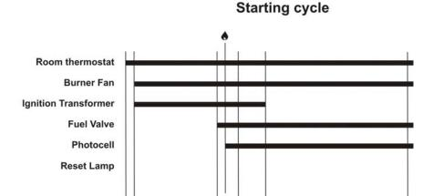
The flame control unit starts the sequence of operation after a heating request (normal operation or thermostat operation) and it consists of the following steps:
