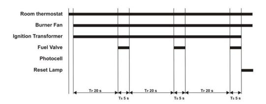
If during the safety time  $T_s$ , the photocell monitors a flame failure (signal to photocell become lower than minimum), at the end of safety time the unit tries to restart twice: should the flame failure being confirmed, then the unit goes in lock out:
