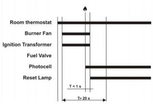
If during the pre-purge time the photocell monitors any residual flame then the unit goes in lock out:
