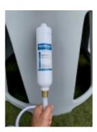
**Step 3** Turn the water source off, then screw the short hose into the top of the filter.
