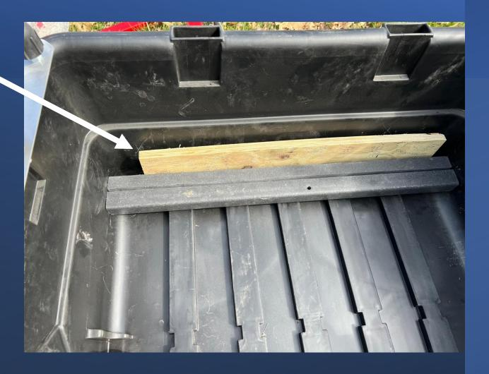
Three boards are fastened from the outside at the ends with two screws in each end.
