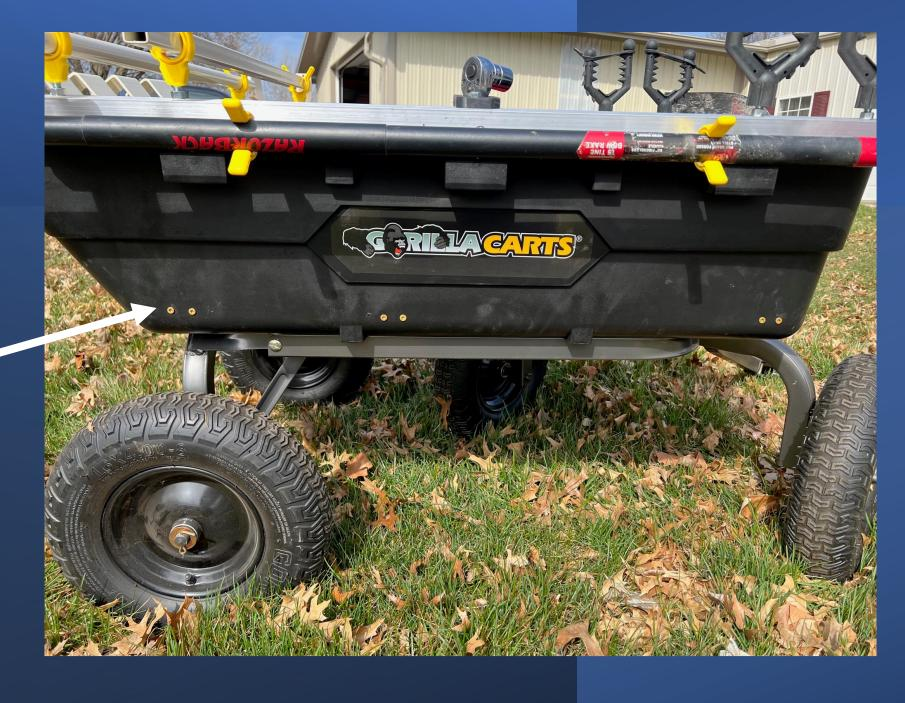
Four lift feet secured in the rubber bump stop assembly here at the back of the angled wagon barrel
