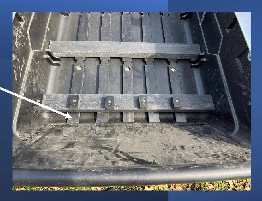
Install Plastic bump and lock board 1 ¾" from angled back of the barrel
