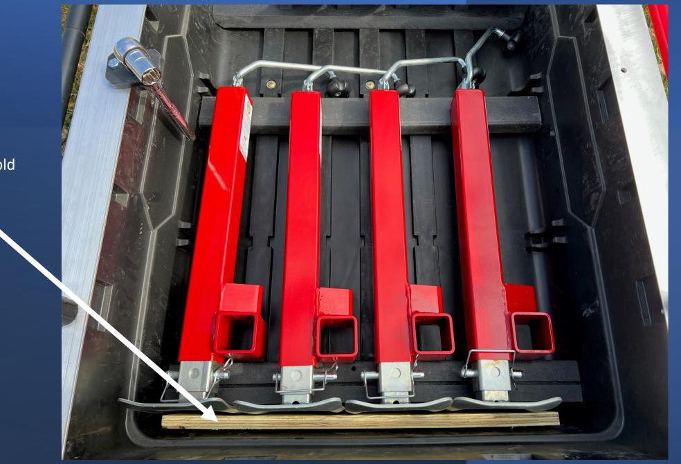
Wood wedge used to hold jacks solid...
