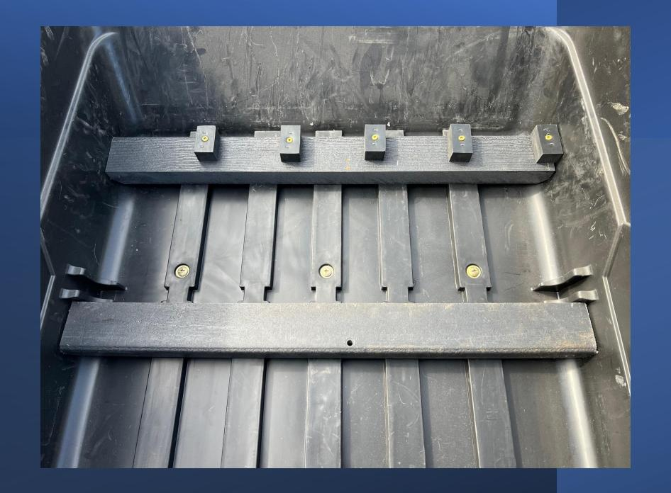
Attach wood screws into plastic boards to secure to the wagon as shown here. 6 on this side and 6 on the opposite side.
