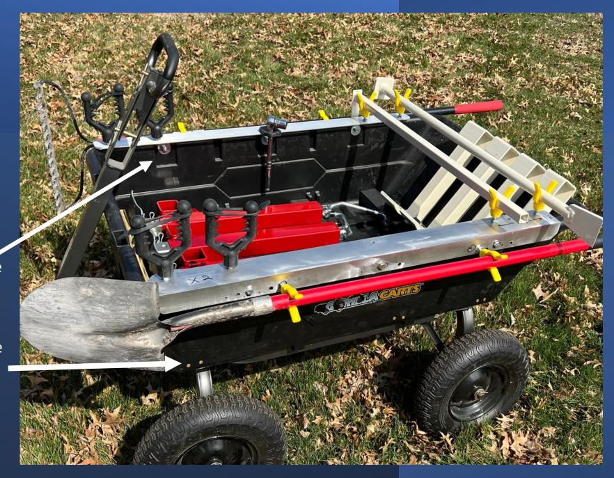
8- Clips to hold shovel, rake, Hoe and digging bar.
