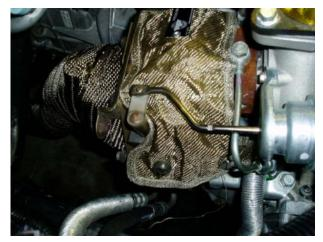
10.) Tie the stainless-steel wire around the rivets exactly the same way you did on the opposite end. Make sure that the blanket fits tightly over the turbocharger.
