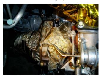
You may re-install your factory heat shield if you desire. Our Subaru turbo blankets can be used in conjunction with or without the factory heat shield.
