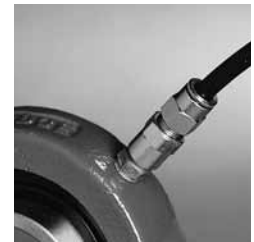
5. And plug the tube into the Quicklinc adapter
