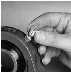
2. Place a Zerk-Lock onto the fitting
