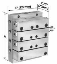
XL Divider Valves are designed to meter large volumes of oil or grease in manual or automatic lubrication systems for all types of industrial machinery. These units can be used in complete XL systems or integrated as a primary divider valve assembly in systems using UV divider valves as secondaries.
