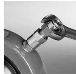
4. Then thread a Quicklinc completely into the Zerk-Lock
