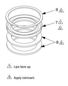
NOTE: Older NXT air motors had one leather seal (8) installed above the u-cup (7). Install new seals as shown above.
