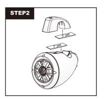
YOU'LL NEED: 3" (76 mm) pads. Remove the backing off the pad and place it in the inner side of both the pod and the mounting bracket.
