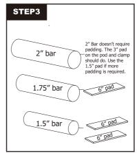
YOU'LL NEED: 6" (150 mm) pads. Remove the backing off the pad and wrap it around the bar.
