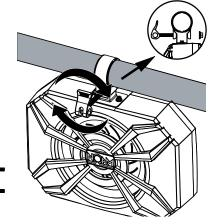
Step 3.1: Push the smart handle to a closed position to tight the mounting band on to the speaker's mounting base.
