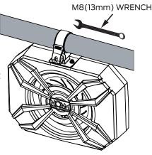
Step 3.2: Using a 13mm nut Wrench, tight the Flange nut for a safe and secure grip of the speaker to the bar.
