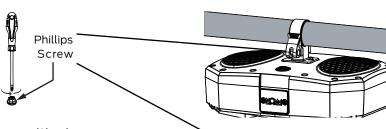
subwooder positioning: using a Phillips screwdriver, you can unscrew the mounting base and screw it back for a monitor position or flat position.
